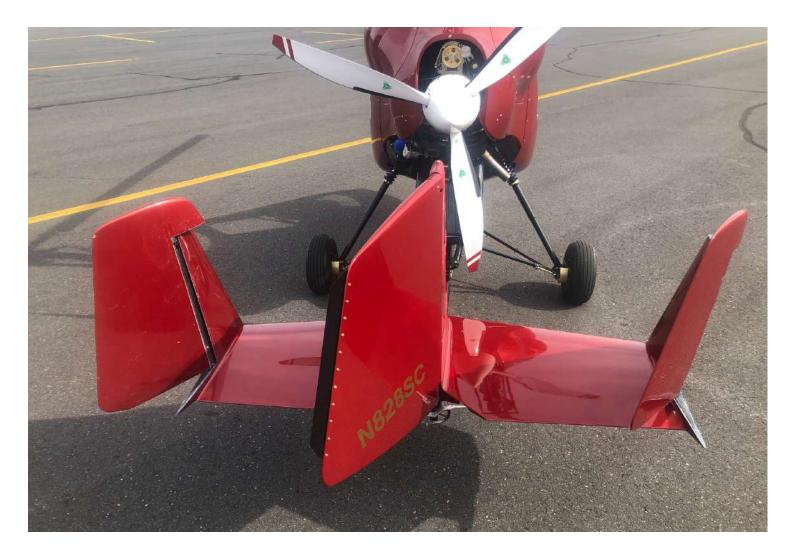
To achieve the best of both mutually exclusive worlds — stability *and* manueverability — required a final modification: a pair of outboard rudders. This is a feature seen only on our SCII, and not on any smaller 2-place gyro.
