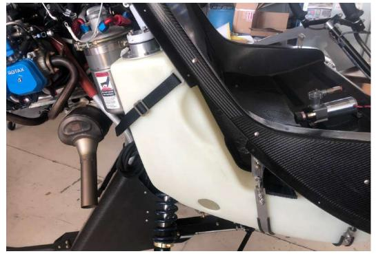
In the M2, you're not sitting directly on top of the fuel tank ,as in other gyros. Rather, the fuel is *outside* the cabin and separated from the occupants by a thick carbon-fiber bulkhead/rollbar with engine firewall layer.
