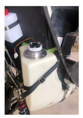
Every Sport Copter M2 has a pair of 11 gallon (usable) rota-molded cross-linked HDPE fuel cells, which feed into an aluminum header tank.
