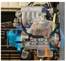
Although rated conservatively on the website, one engine gave 140.6hp @5840rpm, which matches the Rotax 915iS of 141hp for 5 minutes at 5800rpm.
