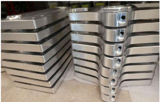
Notice the zerk fittings for the teeter needle bearings – no more lifting out the bar and blades every 25 hours!
