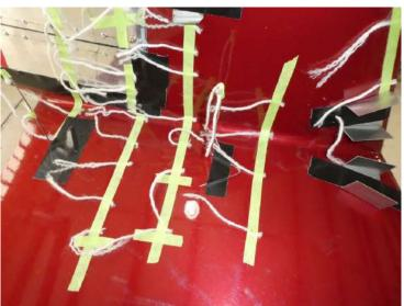
After relentless testing we finally zeroed in on the cause of buffeting, and have increased the airspeed of its onset to now 90+ mph (over 80% of expected  $V_{NE}$ ). So, we know that we're on the right track and will soon eliminate it from the M2 flight envelope. Your Sport Copter M2 will have sure, dependable flight characteristics, with no oddities or surprises.
