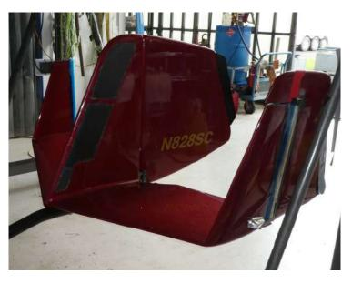
We immediately got the enhanced maneuverability we sought, but with some unexpected tail buffeting at 50+ mph. Solving this took many weeks, and was not easy. We developed several theories, and adapted the outside rudders to test-fly each theory.
