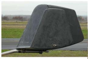
The first M2 carbon tail on its test trailer. First run was up to 80mph, with fine stability.
