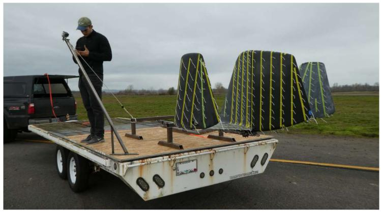
First test of the tufted M2 tail (still shot from GoPro video at ~80mph). Air is evenly hugging the surfaces. Noticeable to us was the aerodynamic force of the tail.
