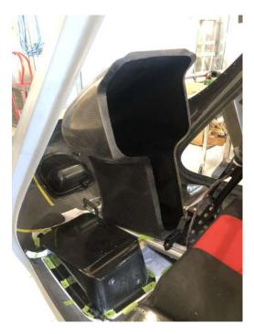
The first large panel has been made, and placed (but not mounted) for position. It's quite large but doesn't much interfere with visibility. It will accept a 10.6" (270mm) glass screen and two airplane sized 1.65" (42mm) high stackable instruments, such as radio and transponder.
