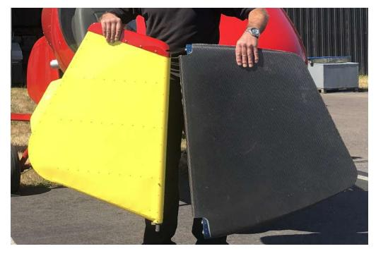
The yellow rudder is from the old M912 to compare with a new M2 rudder.
